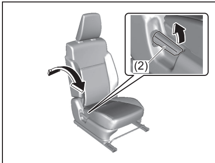
Seatback angle adjustment lever (2) Pull the lever up and move the seatback.
